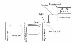
Fig. 1. Schematic diagram of loop coil detector
