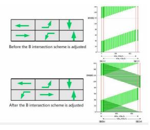
Fig. 7. Comparison chart of coordination effect before and after phase sequence adjustment
